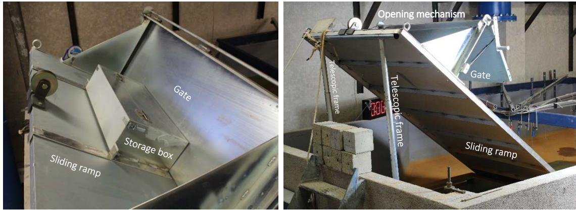
Figure 2. View of the sliding ramp and its accessories.
