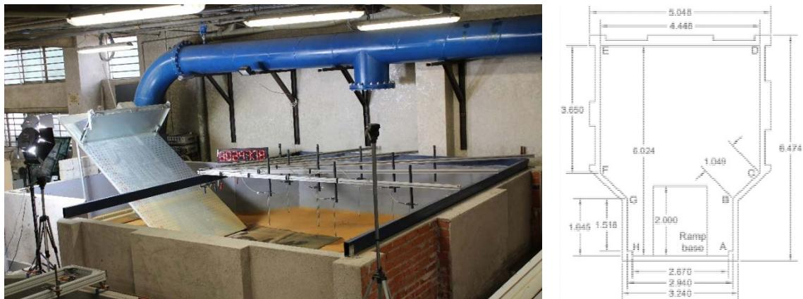
Figure 1. General view of the pool used in the test campaigns (left) and its dimensions in meters (right). The upper conduit in the left image have nothing to do with the facilities used in the experimental campaign.
