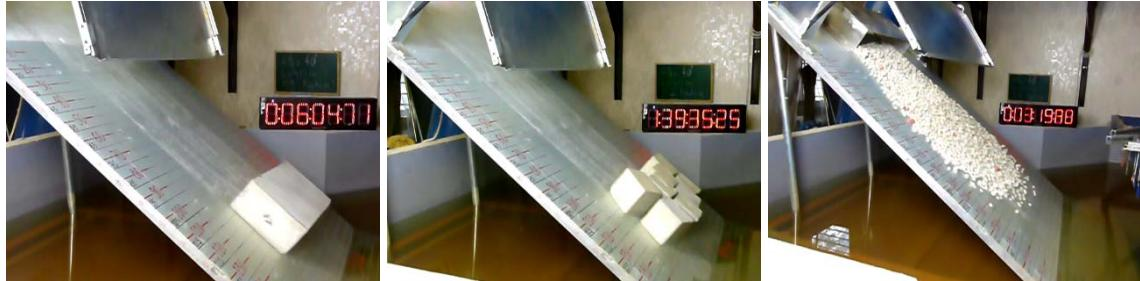
Figure 5. Dispersion along the sliding depending on the material type for  $\alpha = 40^\circ$ . M1 (left), M2 (center) and M3 (right).
