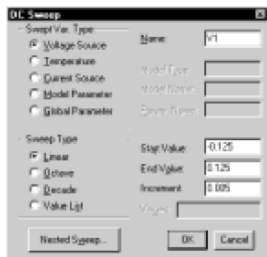
Figure 61 DC Sweep Setup Example
