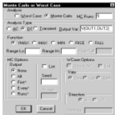
Figure 81 Monte Carlo Analysis Setup for example.sch
