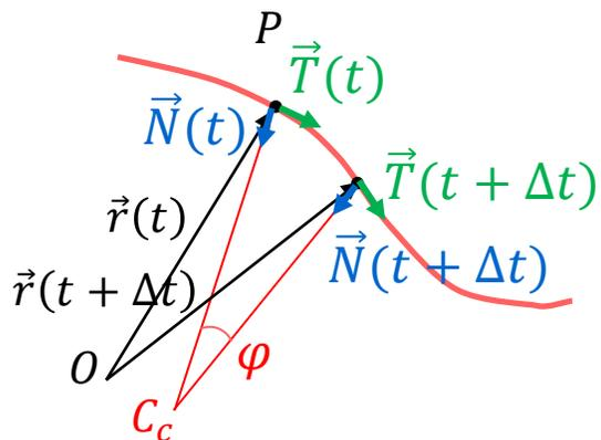
$$\vec{a} = \frac{d\vec{v}}{dt} = \frac{d}{dt}(v \cdot \vec{T}) = \frac{dv}{dt} \cdot \vec{T} + v \cdot \frac{d\vec{T}}{dt} = \frac{dv}{dt} \cdot \vec{T} + v \cdot \frac{d\varphi}{dt} \cdot \vec{N} = \frac{dv}{dt} \cdot \vec{T} + \frac{v^2}{R} \cdot \vec{N}$$
