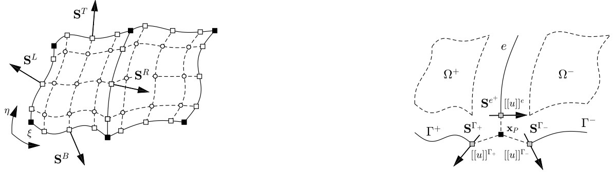
(a) Mappings, curvilinear basis and interpolation nodes. Dashed lines represent \xi = \text{const.} and \eta = \text{const.} according to the curvilinear basis represented. The four normal vectors are a prolongation of \nabla\xi and \nabla\eta lines (orthogonal to the dashed lines). Empty circles represent interior nodes, empty squares represent edge-interior nodes, and filled squares represent edge end-points.
